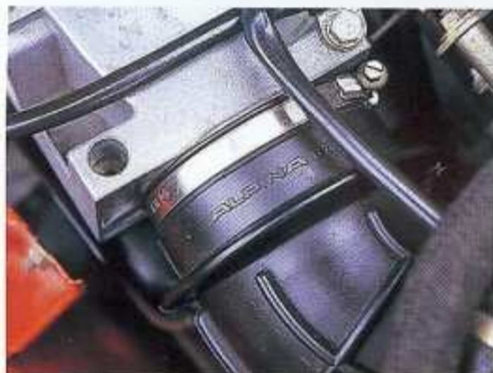
Alpina castings are used to move the intake over to the left to suit the E30.
