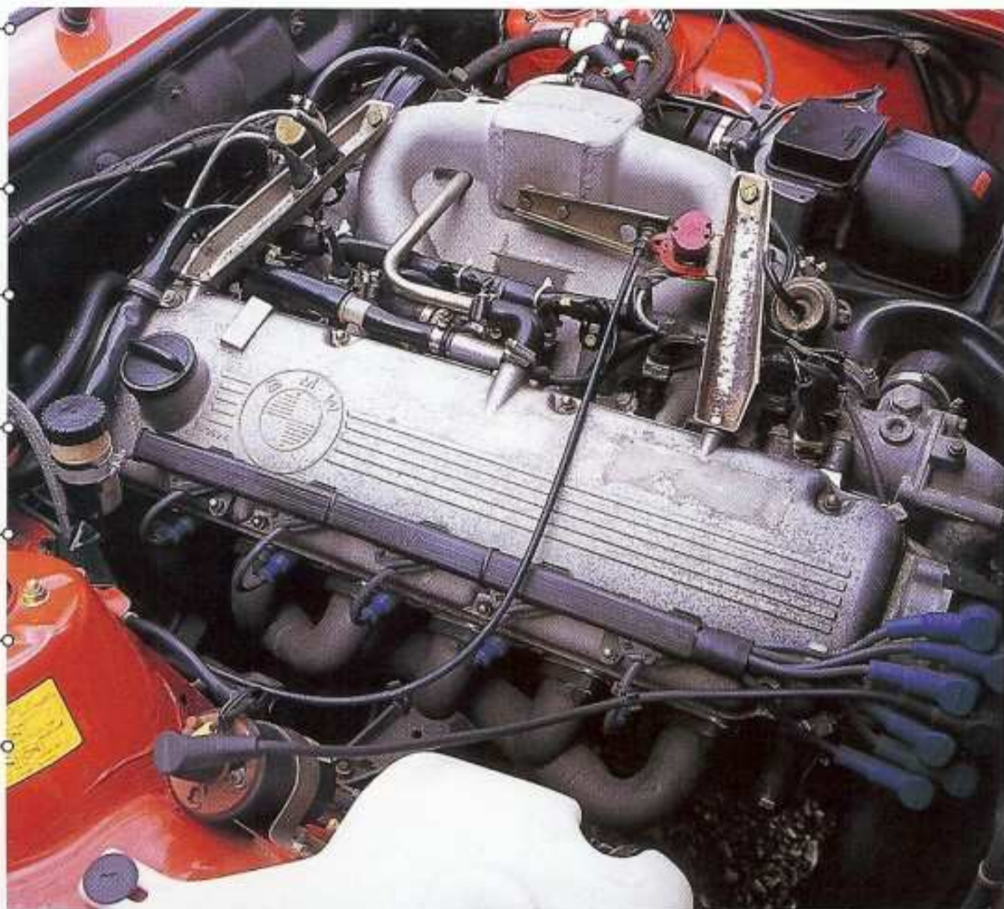
At the 333i's heart is the 3210cc Motronic M30 engine, straight off the production line.
