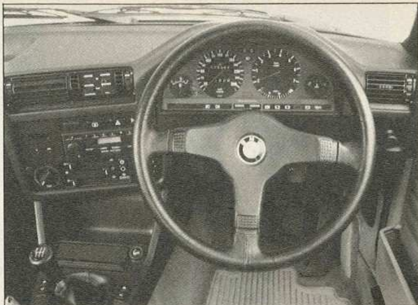
The cockpit is the same as in the 323i (above), except for Alpina instruments which include a 270 km/h speedo and a digital read-out panel mounted in one of the central air vents. The leather-bound wheel is new and the comfortable sports seats (below) are upholstered in leather.
